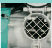
The mixer includes a blocking sensor which detects the opening of the protection grid. Positioned under the covers, the sensor protects the user from accidents, and dust.
